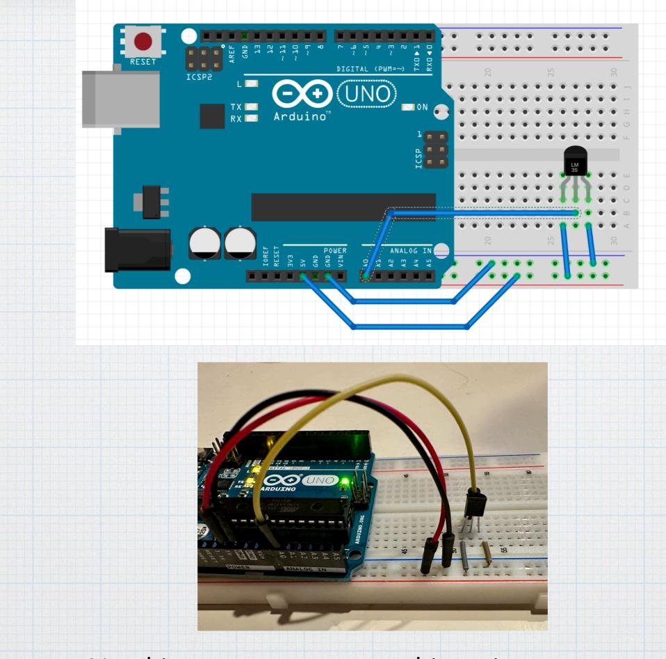
Use this setup to measure ambient air temperature.
