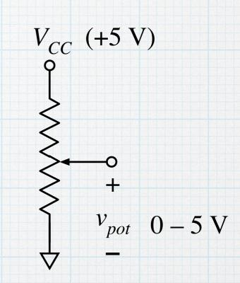
As a simple test, connect the outer leads of a potentiometer to the power supply and ground and the connect to the wiper to to analog input A0. Adjust the potentiometer and print the readings.
