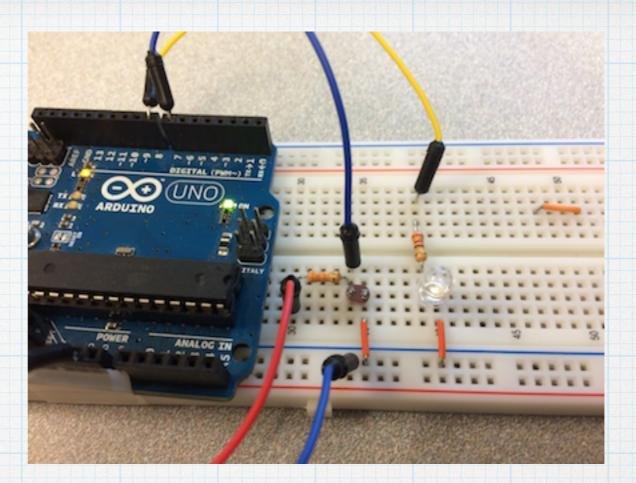
No light hitting the sensor, so the LED is turned on.
