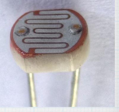
A simple application is to pair a photoresist with a fixed resistor to make voltage divider.
