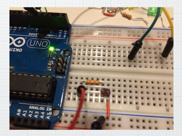
For the photoresistor used here (PDV-9002-1 from Luna optoelectronics, included in EE lab 230 kits), the dark resistance is >150 k $\Omega$ . In typical room light, it measures about 15 k $\Omega$ . Using it with a 33-k $\Omega$  fixed resistor to make a simple voltage divider with a 5-V supply, the dark and light voltages are measured as shown below. The difference between dark and light will be easily discernible using a digital input on the Arduino.
