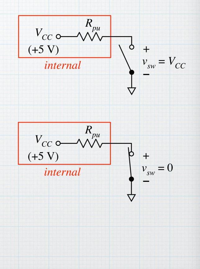
Setup function showing the use of the internal pull-up. The Fritzing diagram shows a momentary switch wired to use the internal pull-up. It couldn't be simpler.
