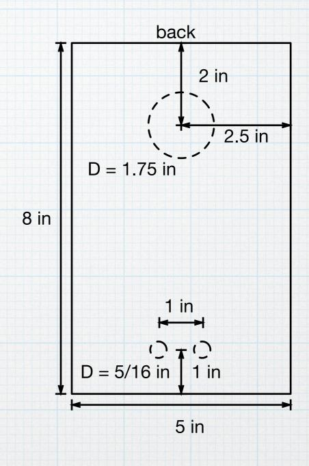
The exact hole locations are not critical. In particular, the tweeter does not need to be offset as shown — since it is sealed, it can go anywhere. Mainly, be sure that holes are not too close to the edges. Also, make certain that the port, which extends inward from the back, does not interfere with the bigger driver, which extends inward from the front — keep one low and the other high. Also note that the fronts should probably be mirror images of each other, if you care about symmetry at all.
