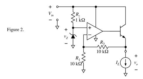
Set up the circuit using a DC supply set to 15 V as the input. Attach a 10-k $\Omega$  resistor as a load and confirm the basic operation by measuring the output voltage. Then perform the following measurements.
