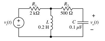
For the component values given, calculate  $f_o$ ,  $Q_P$ ,  $G_o$ , and the bandwidth (in Hz). (Oops, there's a clue in there.)
