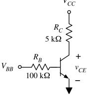
a. Find the DC values for  $i_C$  and  $v_{CE}$  for the following power supply combinations. Also, calculate the values by hand using the simplifying forward-active and saturation models for the BJT. You should use a *bias point* simulation for these DC calculations.
