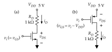
Then, during your turn with the parameter analyzer, measure a set of  $i_D - v_{DS}$  curves for one NMOS transistor and one PMOS from the CD4007 array and also for the IRF540 power NMOS Then, using the same transistors, obtain plots of  $i_D^{1/2}$  vs  $v_{GS}$  and use that to determine  $V_T$  and K for the transistor. Take photos of the curves to include in your report.
