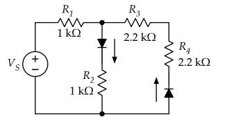
Figure 4. Find the currents in both diodes and all three resistors.
