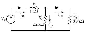
Figure 3. Do this first with  $V_S = +5$  V. Then repeat with  $V_S = -5$  V.
