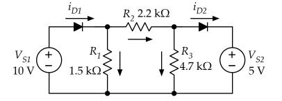
Figure 5. Find the all of the indicated currents. Do this first for  $V_S = +1$  V, and then repeat for  $V_S = +5$  V.
