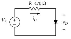
The repeat the measurement using the 1N7433 Zener diode over the same range.
