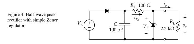
Repeat all the measurements from part C. (Different load resistance and different source amplitudes.) Note that it may be difficult to measure the ripple voltage using the oscilloscope, because the ripple should be much smaller. (Of course, this is the point in using the regulator circuit.) Record the ripple and the average voltages measured using the meter.
