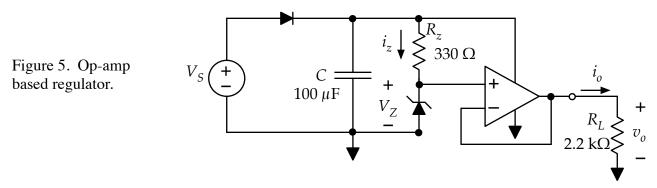
The op-amp is in the unity-gain configuration, so the output voltage should be equal to the Zener voltage.
