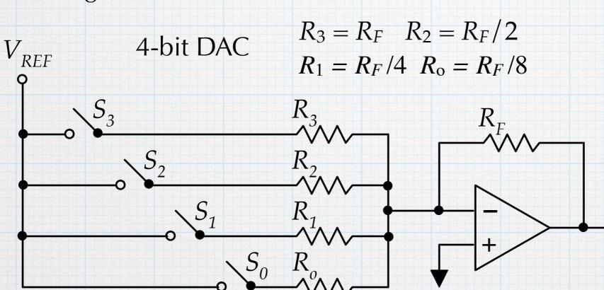
The digital bits control the operation of the switches – one bit per switch.  $S_i = 0$ , switch is open,  $S_i = 1$  switch is closed.  $S_o$  only closed:  $v_o = -V_{REF}/8$ .  $S_1$  only closed:  $v_o = -V_{REF}/4$ .  $S_2$  only closed:  $v_o = -V_{REF}/2$ .  $S_3$  only closed:  $v_o = -V_{REF}$ . Combinations of switched will be summed, and the scaling EE 230 matches that of a digital number.
