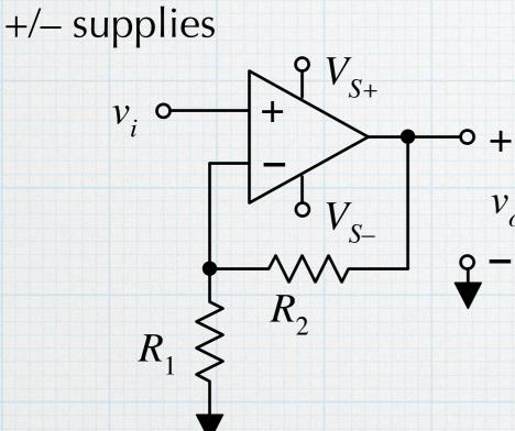
And most often, we ignore even the power supply connections, simplifying the circuit diagram further. (However, we must be aware of the power supplies being used, because they will affect the performance of the op amp.)
