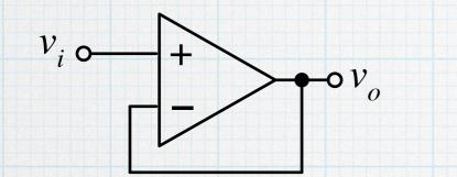
Non-inverting amp with  $R_2 = 0$  and  $R_1 \rightarrow \infty$ . So G = 1, meaning  $v_o = v_i$ . This seems a bit dumb. What good is it?
