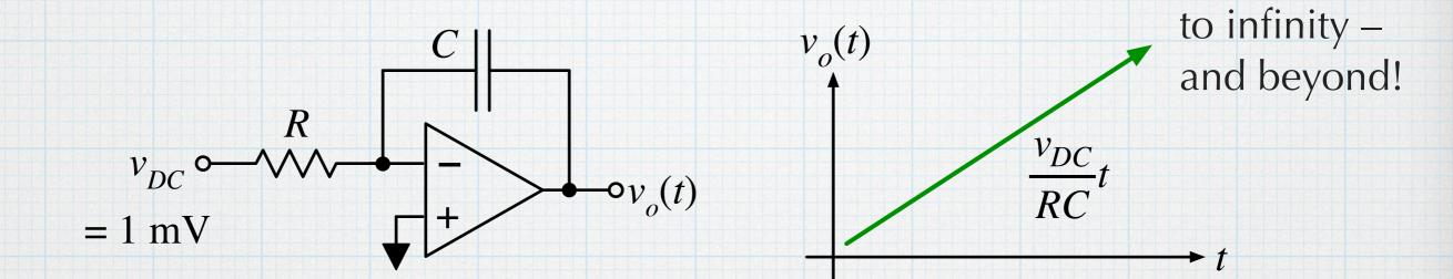
This is a problem because at DC, the capacitor is an open circuit and the amplifier has essentially infinite DC gain. To make it better, put a resistor in parallel with the cap,  $R_2 >> R_1$ . This limits the DC gain to  $-R_2/R_1$ .
