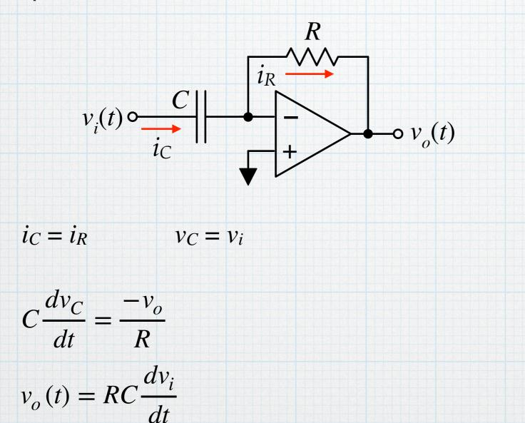
However, differentiating amps are not used much. If there is noise at the input (characterized by random, fast variations), the differentiator tends to make it worse. The integrator, on the other hand, tends to average out the effects of noise.
