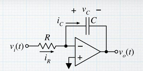
$$v_o(t) - v_o(0) = -\frac{1}{RC} \int_0^t v_i(t') dt'$$
