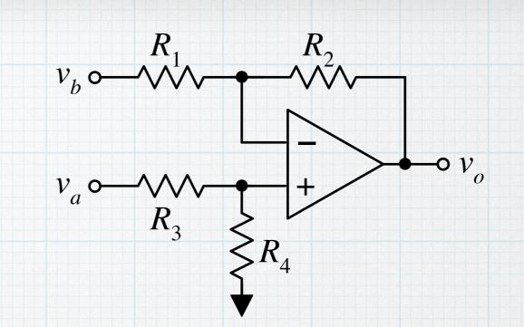
But it could be better. First, the input resistances seen by  $v_a$  and  $v_b$  depend on the values of  $R_1$  and  $R_3$ , which might be smallish. (See earlier slide on input reistance. Secondly, it might be nice to be able adjust the gain using a potentiometer, but that is difficult because of the requirement that ratios be matched.
