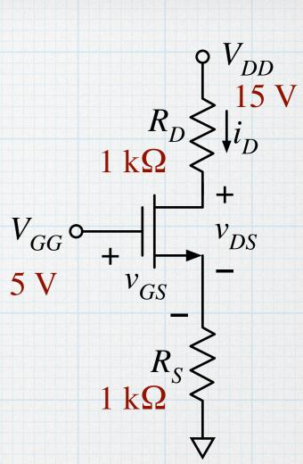
To help decide the issue, we could *guess* that the transistor is off, meaning that we are assuming  $v_{GS} < V_T$ . However, if the NMOS is off, then  $i_D = 0$ . This makes  $v_{GS} = V_{GG} - i_D R_S = V_{GG} = 5$  V. This is greater than  $V_T$ , meaning that the transistor should be on — in exact contradiction to the assumption of the transistor being off. So the transistor must be on.
