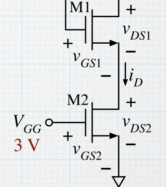
$$K_{n1} = \frac{1}{2} \mu_n C_{ox} \frac{w_1}{L} = 0.1 \frac{\text{mA}}{\text{V}^2} \text{ and } K_{n2} = 0.4 \frac{\text{mA}}{\text{V}^2}.$$
