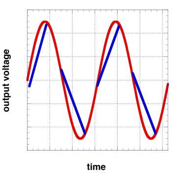
Even though the slew rate imposes a frequency limit for sinusoidal signals, it is fundamentally different than the gain-bandwidth. Slew rate limits will distort the signal. The bandwidth limitation will give an undistorted signal, but with a possibly reduced amplitude.
