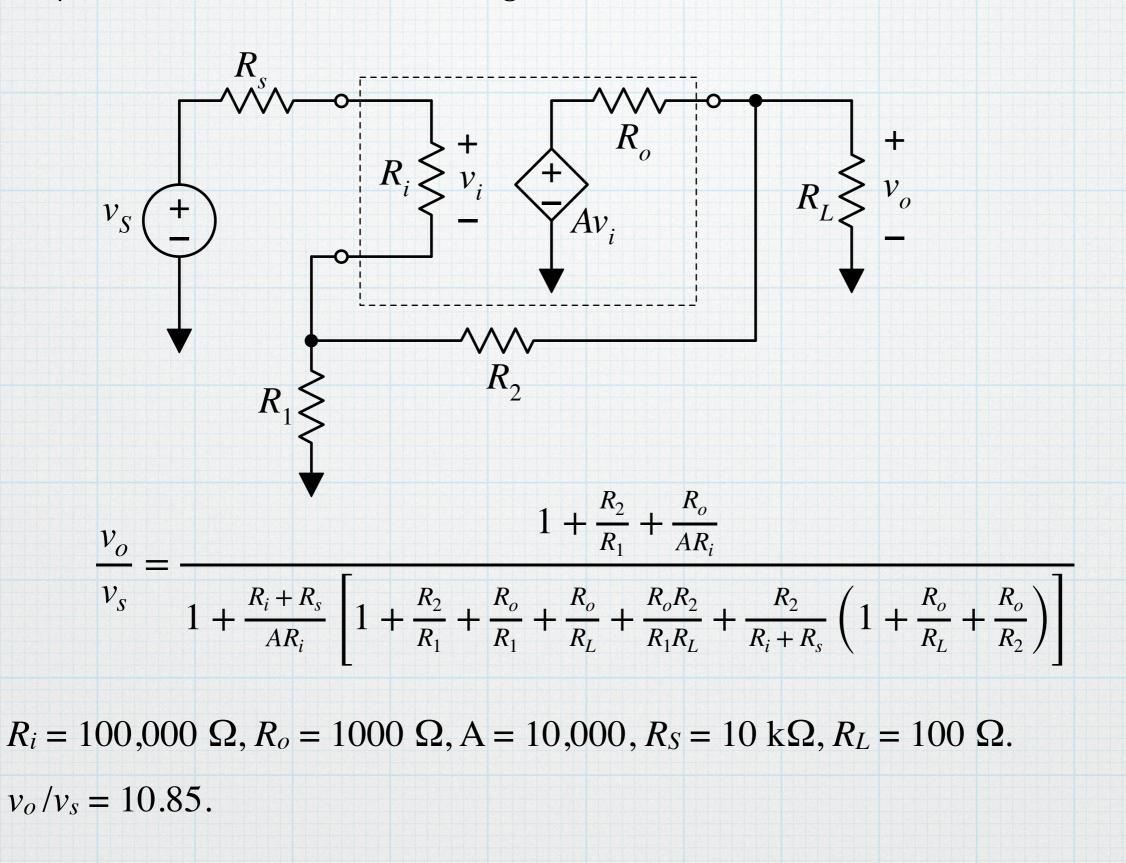
$$R_{o} = 0 \qquad \frac{v_{o}}{v_{s}} = \frac{1 + \frac{R_{2}}{R_{1}}}{1 + \frac{R_{i} + R_{s}}{AR_{i}} \left[1 + \frac{R_{2}}{R_{1}} + \frac{R_{2}}{R_{i} + R_{s}}\right]}$$
