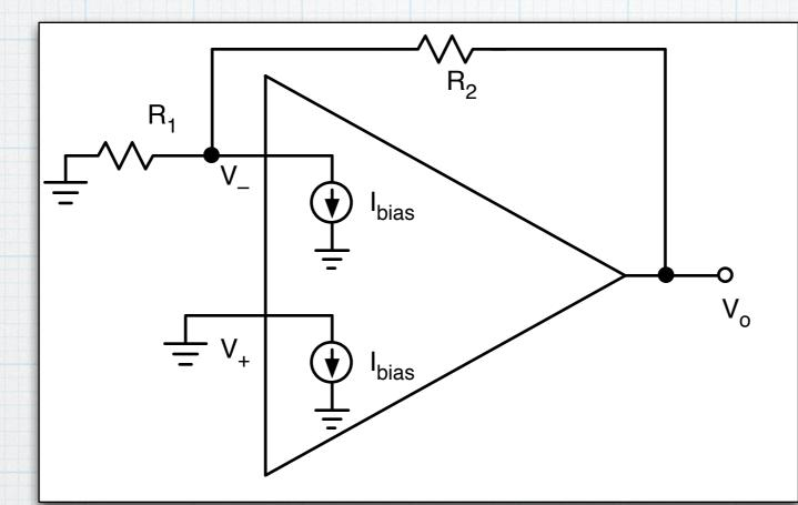
Using virtual ground:  $V_{-} = V_{+} = 0$ .
