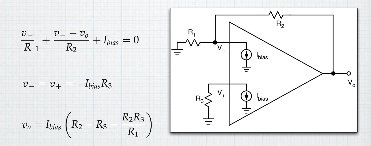
The output will be zero, if we choose  $R_3 = R_1 || R_2$
