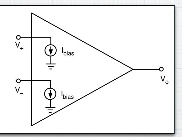
To see the effect of the bias current, hook up an inverting amp.
