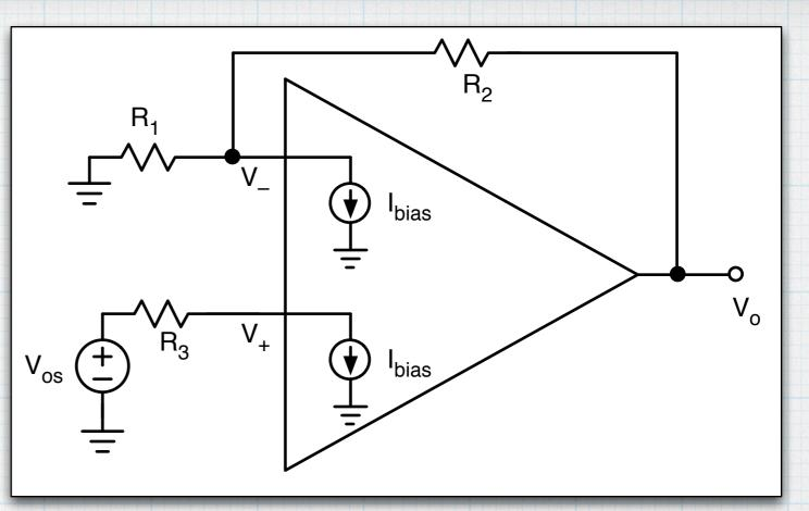
Use superposition (or solve node voltages from scratch, as done below) to see the cumulative effect.
