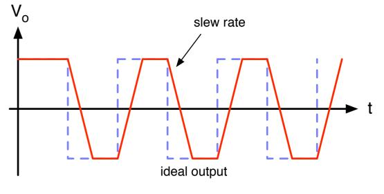
Although slew rate limits are most evident with square-wave transitions, they can affect any waveform. Consider a sinusoid at the output:  $v_o(t) = V_m \cos(\omega t)$ .
