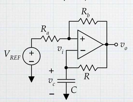
1. Suppose that the input is low and the output is high. The capacitor voltage is also low. 2. The output voltage will charge the capacitor.
