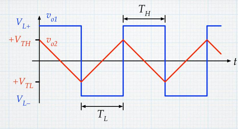
The output of the comparator will be a square wave, with high and low voltages given by the output limits and high and low times determined by the specifics of the hysteresis curve and the RC time constant of the integrator.
