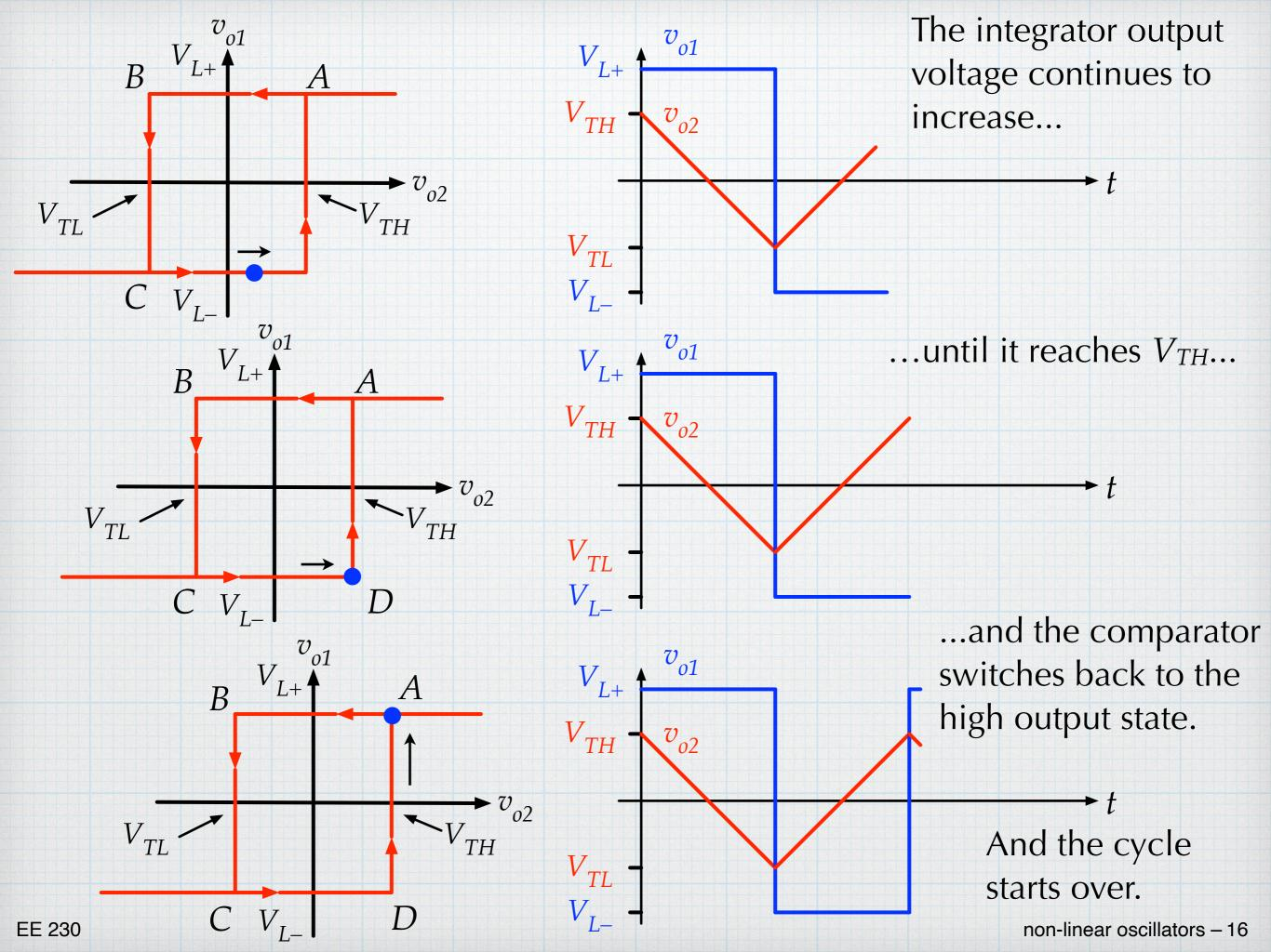
The total period of the oscillation will be determined by the time needed for the integrator to ramp up and down between  $V_{TL}$  and  $V_{TH}$ . This is represented by the times needed to move across the top and bottom of the transfer characteristic.
