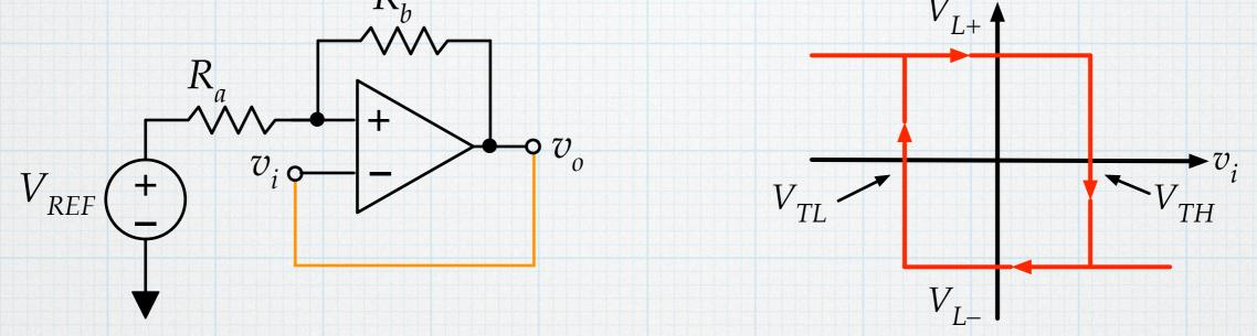
$V_{TL}$  and  $V_{TH}$  are given by the expressions derived in the comparator notes. Fiendish question: What would happen if we tied the output back to the input?
