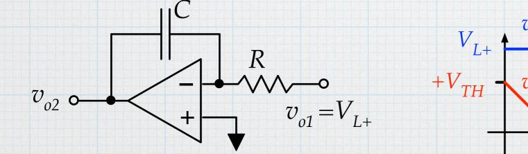
$$v_{o2}\left(t\right) = V_{TH} - \frac{V_{L+}}{RC}t$$
