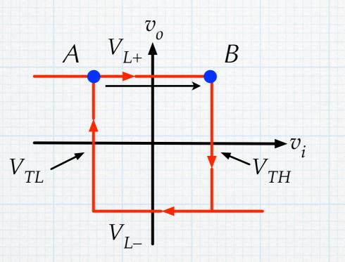
The time required to move from *A* to *B* on the characteristic is found using the capacitor charging equation. This is the time that the output will be high.
