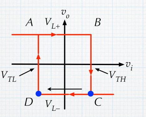
Again, the time required to move from *C* to *D* on the characteristic is found using the capacitor (dis)charging equation. This is the time that the output will be low.
