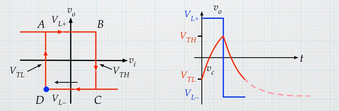
...which causes the comparator to switch abruptly to the high-output condition – right back to where we started.
