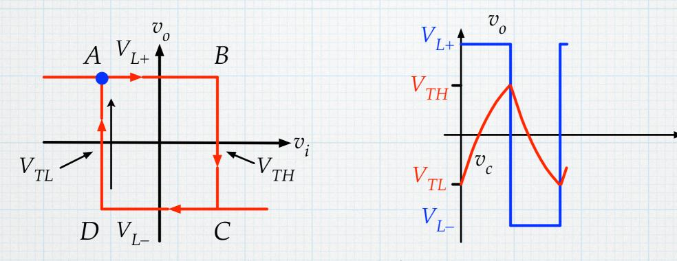
The cycle starts over and repeats indefinitely. The capacitor charges and discharges between  $V_{TH}$  and  $V_{TL}$  and the output switches between  $V_{L+}$  and  $V_{L-}$ .
