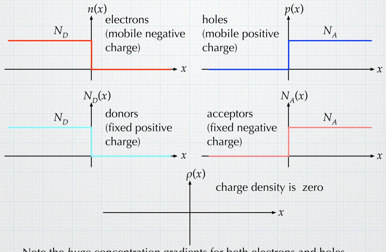
Note the *huge* concentration gradients for both electrons and holes. Both will start to diffuse — electrons to the right and holes to the left.
