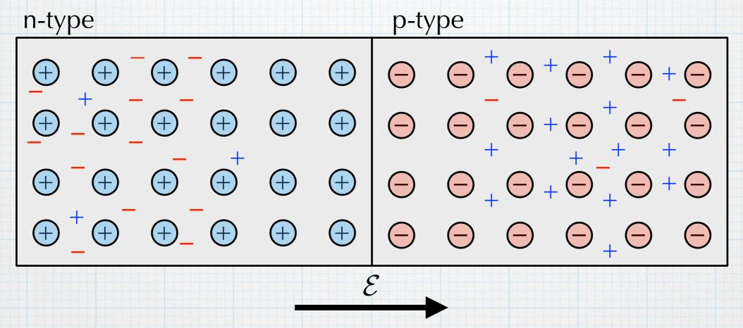
As the carriers diffuse across the junction, creating the space-charge layer, the electric field builds up.
