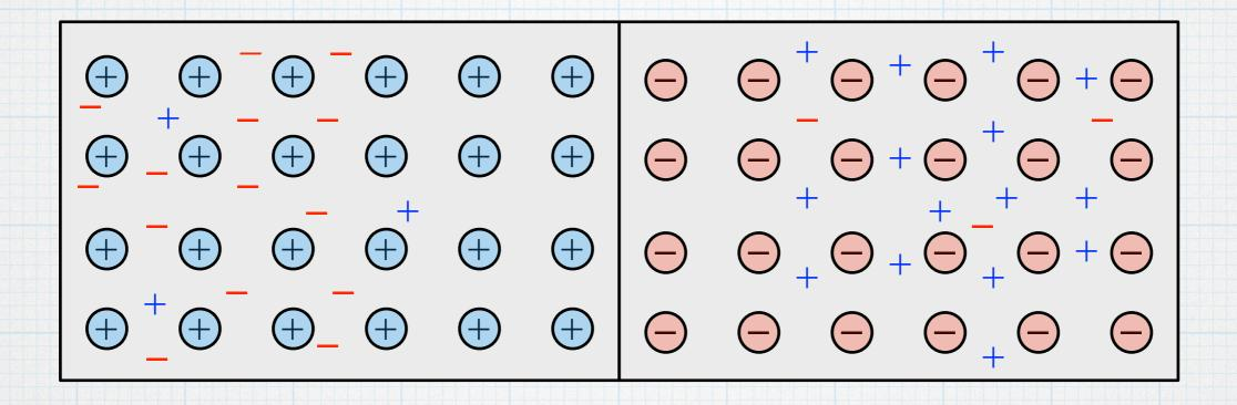
Around the junction, the net charge is no longer zero!
