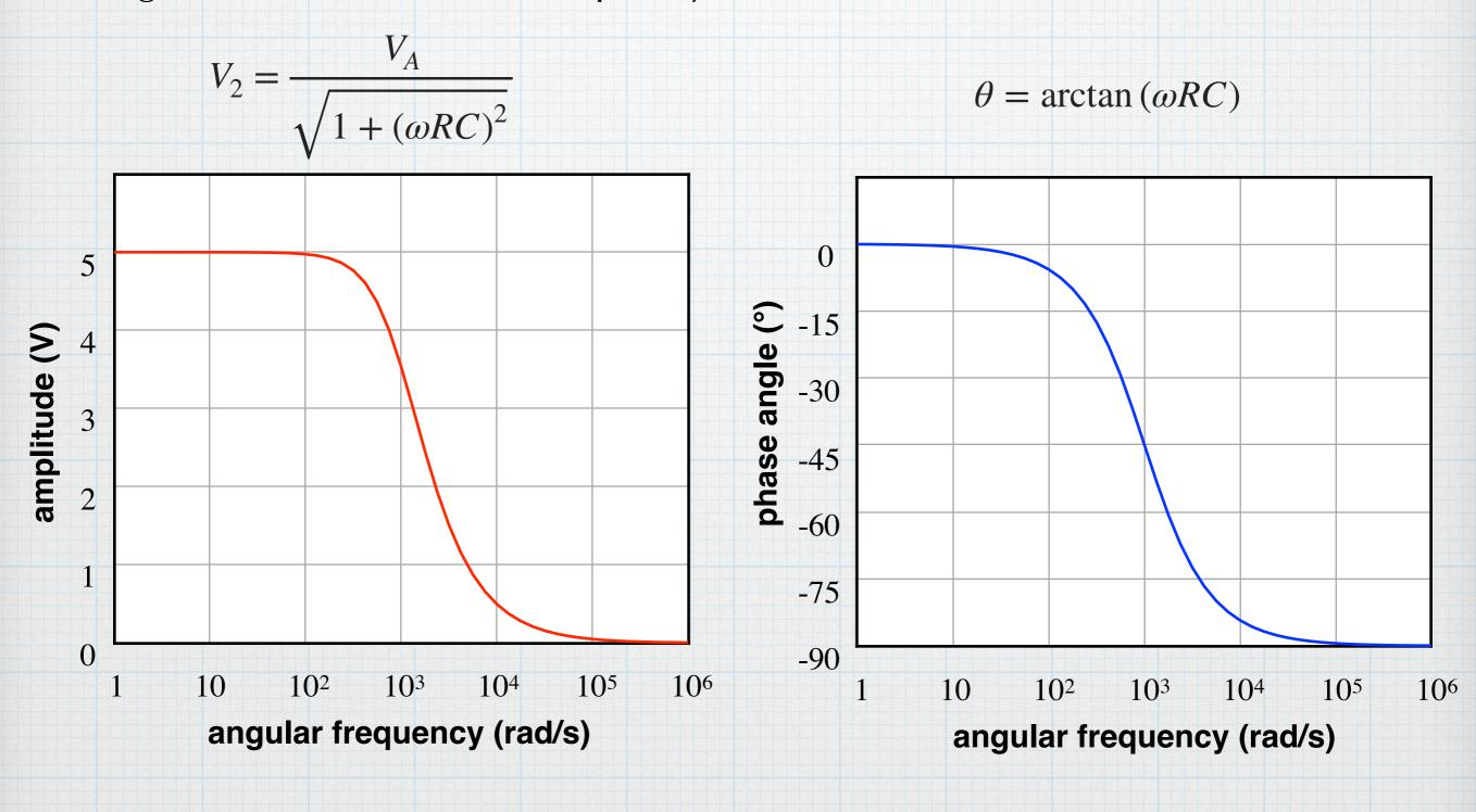
The plots bear out the features of the amplitude and phase functions.
