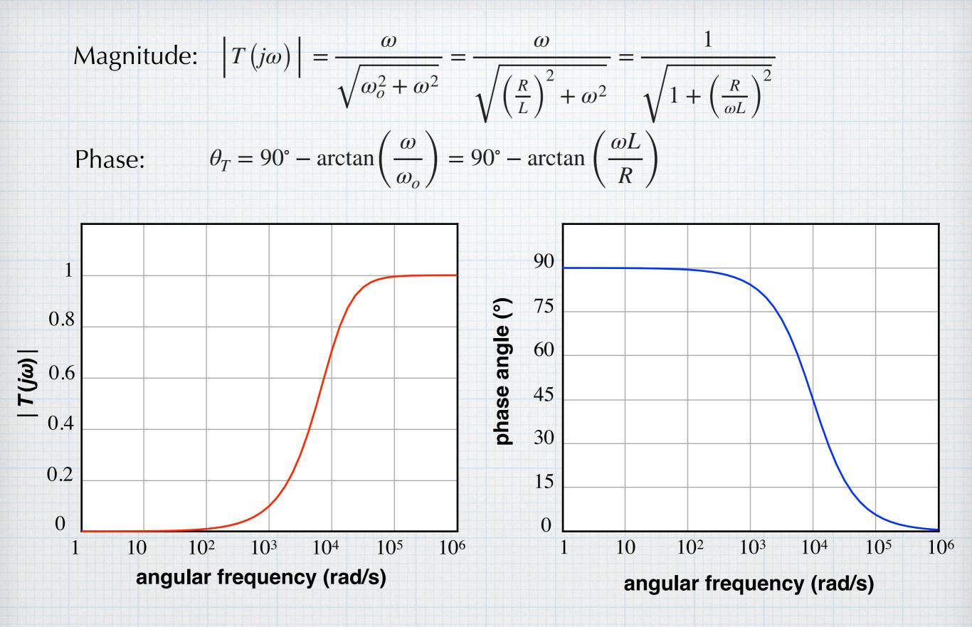
This one has a different behavior. It starts low at low frequencies and the magnitude increases as the frequency increases.
