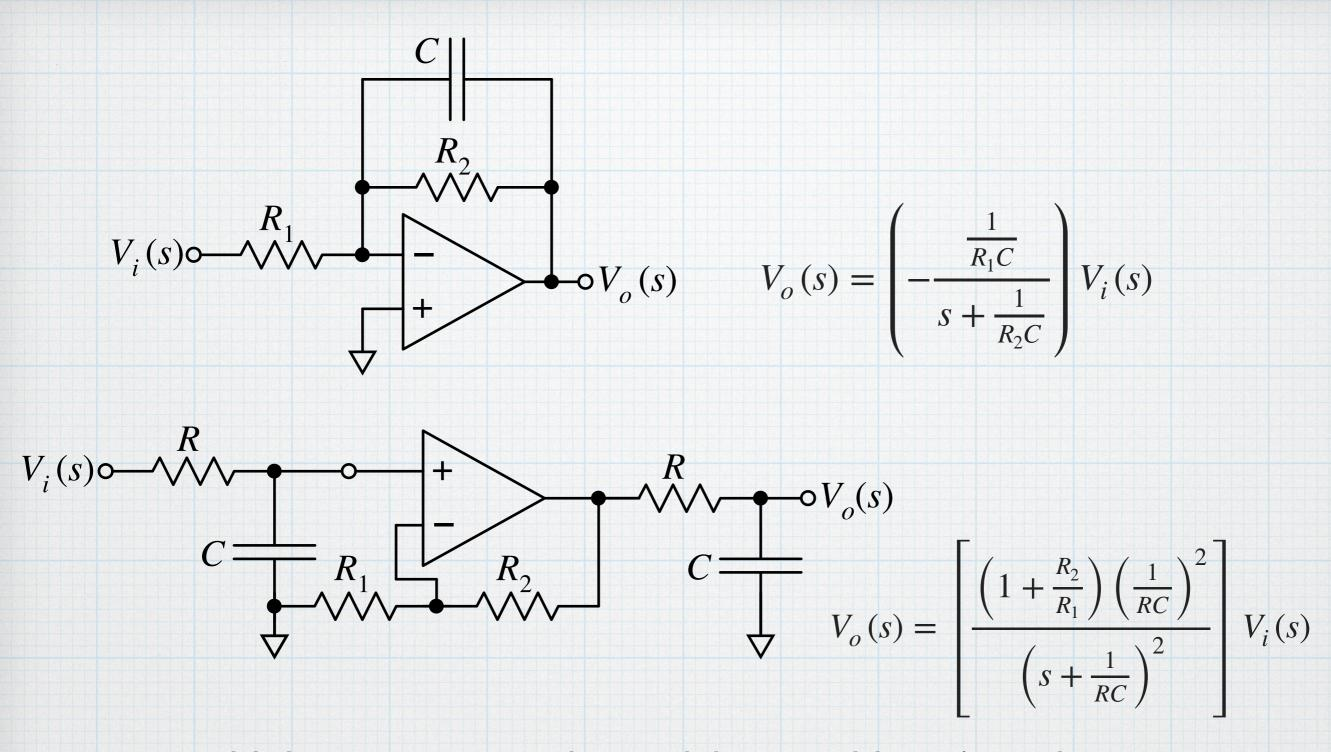
We could show more examples, and they would reinforce the pattern that should be clear — when finding a voltage or current in the frequency domain, the result will always be in the form of a function that is derived from the circuit, multiplied by the Laplace transform of the source. The frequency-domain expressions in the previous circuit examples could be generalized to a simple form:
