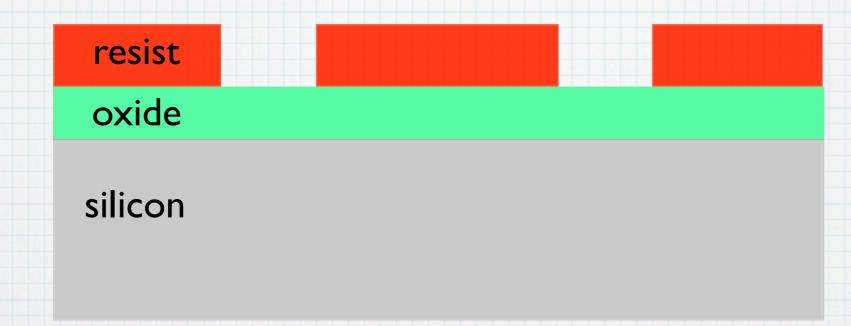
Immersing everything into the developer removes the exposed resist. The developer does not affect the masked photoresist (as long as the wafer is not left in the developer too long.) The developer does not affect the silicon or the oxide. The photoresist serves as a masking layer for etching into the oxide. An acid etch is used to remove the oxide in the exposed regions, transferring the pattern to the oxide layer.
