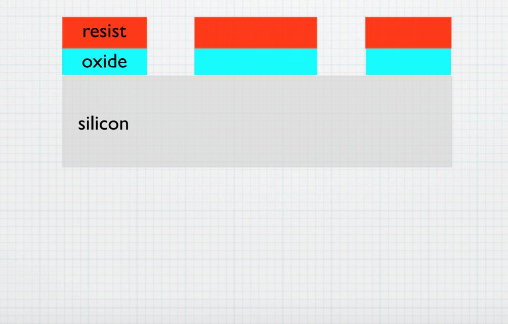
Finally, the photoresist is washed away using a simple solvent, like acetone (finger-nail polish remover). The wafer, with the patterned oxide, is ready to go on to the next step in the process.
